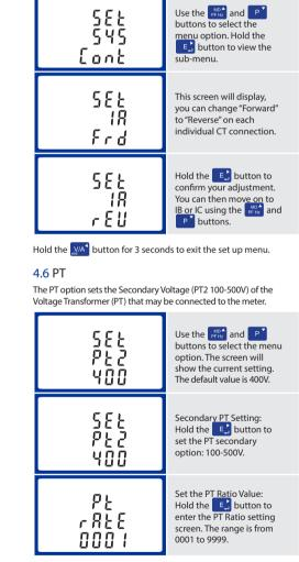
The PT Rate is the PT Primary divided by the PT Secondary. For Example: Voltage Transformer - 11000÷110=100, so the PT Rate would be 0100 and the PT2 would be 110.
