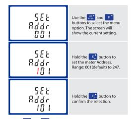
Use the 100 and P buttons to choose the necessary number, then press the D button to move along to the next number. To save the new setting, hold the D button for 3 seconds until the selection stops flashing
