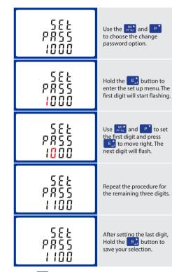
Hold the 💹 button for 3 seconds to exit the set up menu.
