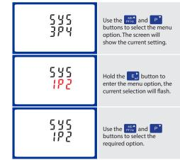
Hold the E button to confirm your adjustment. Hold the button for 3 seconds to exit the set up menu.
