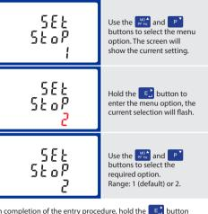
On completion of the entry procedure, hold the E for 3 seconds until the selection stops flashing
