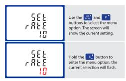
Use the price and price buttons to choose the desired pulse rate. To save the new setting, hold the circle button for 3 seconds until the selection stops flashing
