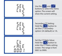
The CT Rate is the CT Primary divided by the CT Secondary. For Example: 200/5A Current Transformers - 200÷5=40, so the CT Rate would be 0040 and the CT2 would be 5.
