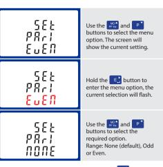
On completion of the entry procedure, hold the 💽 button for 3 seconds until the selection stops flashing
