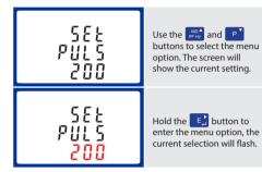
Use the part and P buttons to choose the desired pulse rate. To save the new setting, hold the E, button for 3 seconds until the selection stops flashing.
